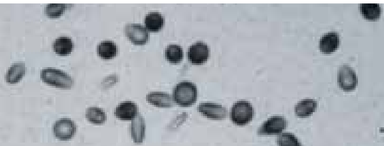
Microphotograph of particle tracks in CR-39 material from 222 Rn decay. Courtesy of INFN Bologna.
